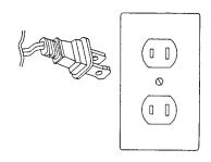
fail to fit, contact a qualified electrician to replace the obsolete outlet. Do not defeat the safety purpose of the polarized plug.
